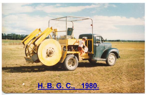
Double drum used at Roys Hill strip next to river, 4.5 air miles from Bridge Pa. Over one mile wire on each drum. Best launch height, 2.200 Ft for K6 CR.
